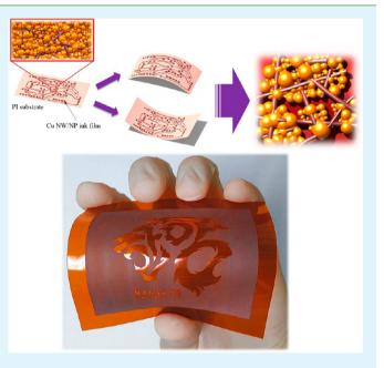
NW/NP ink film, X-ray diffraction and scanning electron microscopy were used. KEYWORDS: flash light sintering, copper nanoparticles, copper nanowires, printed electronics, reliability of electrode
